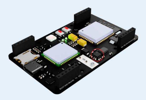
On the Micromis Base VI development board is the MPU6050 chip, which can read acceleration and spatial orientation - a combination of a gyroscope and accelerometer.
