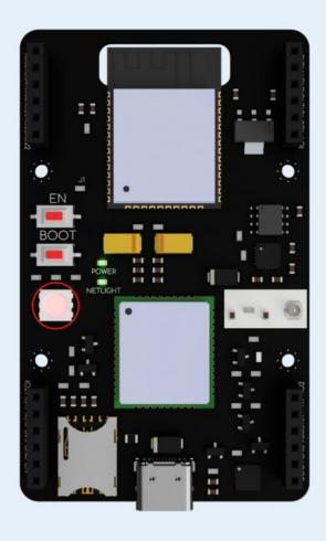
The Micromis Base VI development board is also equipped with an addressable RGB LED to emit light signals. The mounted diode includes the WS2812C chip, which controls the diode and allows the user to select the color and color saturation for the diode's light. Due to the use of RGB technology, there are more than 16 million combinations at the user's disposal to achieve satisfying lighting effects.
