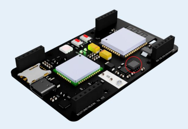
In addition to the MPU6050 chip, an LM75 temperature sensor is mounted on the Micromis Base V1 development board, which allows reading ambient temperatures from -55  $^{\circ}$ C to +125  $^{\circ}$ C.
