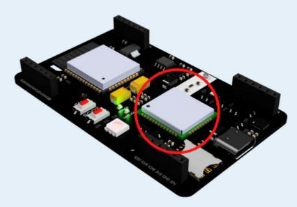
The Micromis Base VI development board has a built-in Quectel M65 modem for GSM network communication, which allows the device to connect to the Internet without WiFi and send SMS messages.
