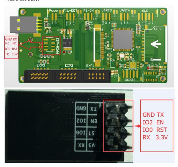
Connection method: Use the DuPont line to connect to the Pin.
