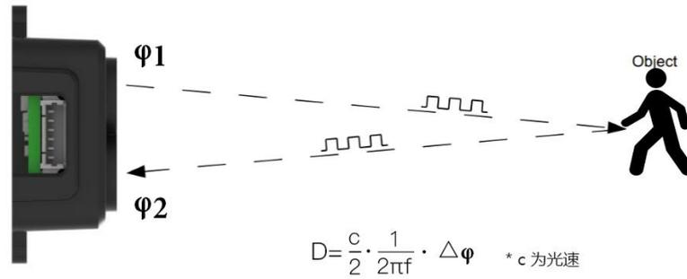
*Figure 1: Schematics of TOF Principle*
