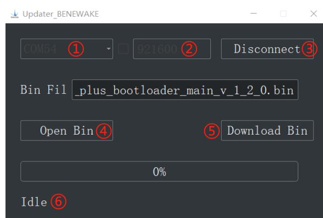
Figure 6: Firmware Upgrade PC software of TF-Luna
