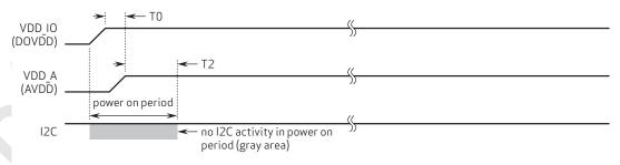
$\begin{array}{l} \textbf{note} \quad T0 \geq 0 \text{ ms: delay from VDD}\_10 \text{ stable to VDD}\_A \text{ stable} \\ T2 \geq 1 \text{ ms: delay from VDD}\_A \text{ stable to sensor power up stable} \end{array}$
