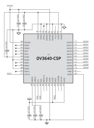
note 1 JPI STROBE AGND SIOD 3 AVDD 4 SIOC RESETB 6 VSYNC PWDN 8 HREF 9 FREX 10 DOVDD 11 DATA9 12 XCLK 13 DATA8 14 DGND 15 DATA7 16 PCLK 17 DATA6 18 DATA2 19 DATA5 20 DATA3 21 DATA4 22 DATA1 23 DATAO 24
