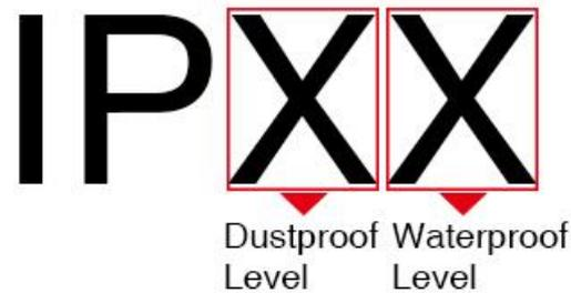
TF03 has its protection level of IP67 - IP dust proof level 6, IP waterproof level 7.
