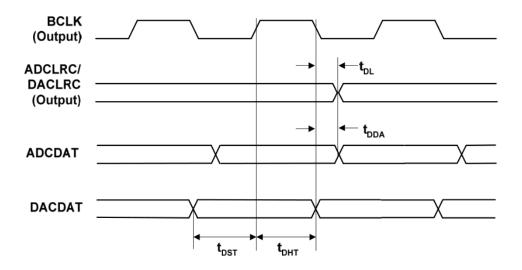
I2S has four signal lines, they are: SCLK, LRCK, SDATA and MCLK. And the first three are most important. For better synchronize with system clock, you can mater device clock, or external clock circuit.
