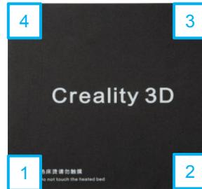
3. Move the nozzle to the front/left leveling screw and adjust the platform height by turning the knob underneath. Use a piece of A4 paper (standard printer paper) to assist with the adjustment, making sure that the nozzle lightly scratches the paper.
