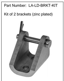
This bracket is tested to 703 lbs., which is 125% of the highest static load that Concentric International's Light Duty line of actuators are rated for.
