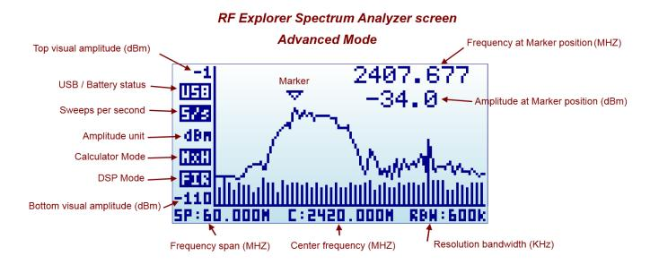
Note the frequency axis indicators changes at the bottom. More details about this screen mode in section *Analyzer screen* page 16.
