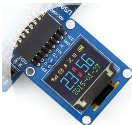
Figure 1: OLED information display
