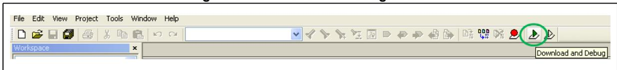
6. The debugger in IAR Embedded Workbench® can be used to debug source code at C and assembly levels, set breakpoints, monitor individual variables and watch events during the code execution.
